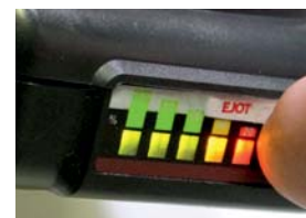
External visual charge indicator on each battery.
