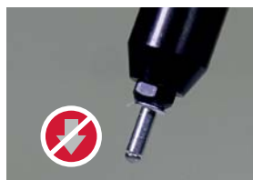
Retention nose pieces prevent the falling out of the rivets in a vertical position.
