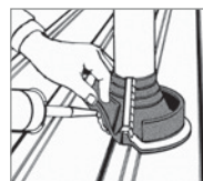
4. Apply sealant and fit Dektite® accurately to the profiled sheet.
