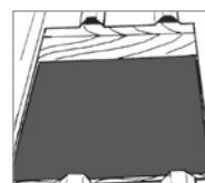
4. Cut out the roof inside of the marked 30 mm area. Trim sharp edges. Timber supports may be installed to support the roof where ribs have been removed.
