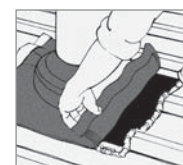
5. Apply sealant and fit Dektite® accurately to the profiled sheet.
