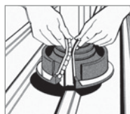
2. Place the Dektite® around the pipe and engage metal teeth in opposing pockets starting at the top.
