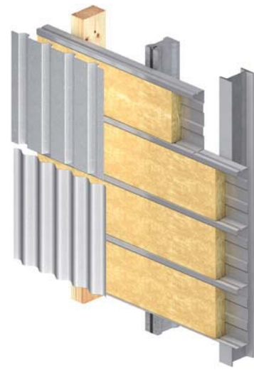
Profiled wall with cassette structure Page 34
