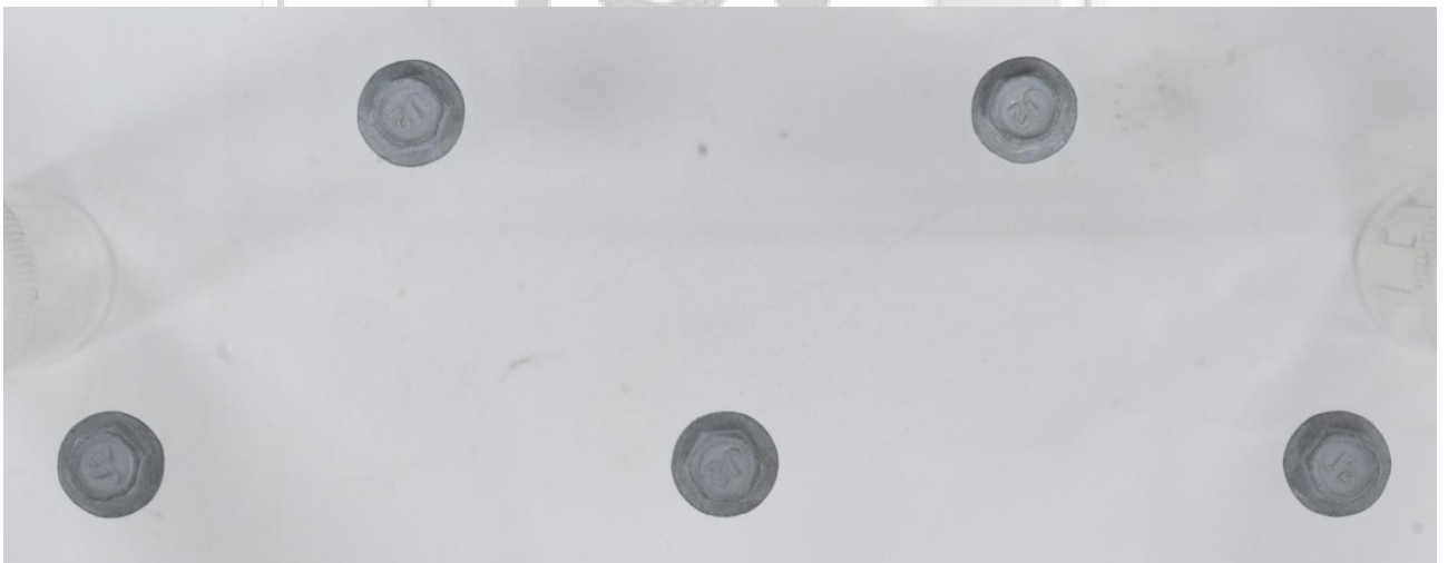
Figure 2. After 1,000 hours of water resistance test in 100% relative humidity
