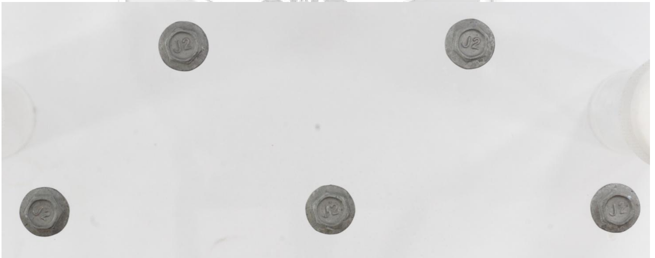
Figure 2. After 15 cycles of exposure in condensing atmosphere containing sulphur dioxide
