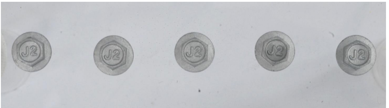
Figure 3. After 1,000 hours of Cyclic Fluorescent UV Lights and Water Condensation Test
