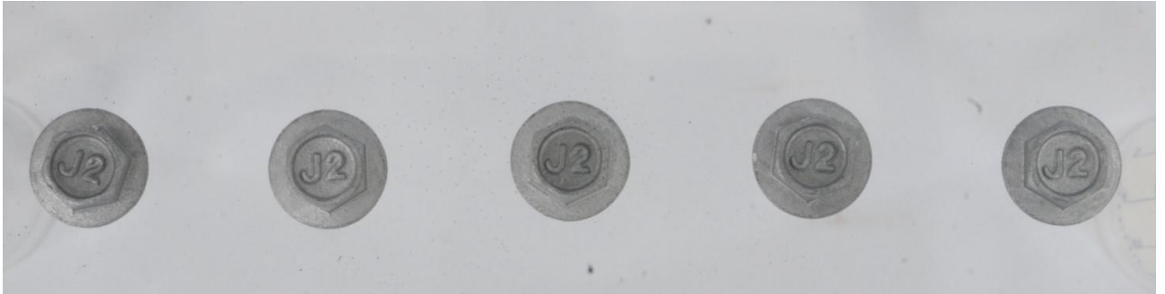
Figure 4. After 1,500 hours of Cyclic Fluorescent UV Lights and Water Condensation Test
