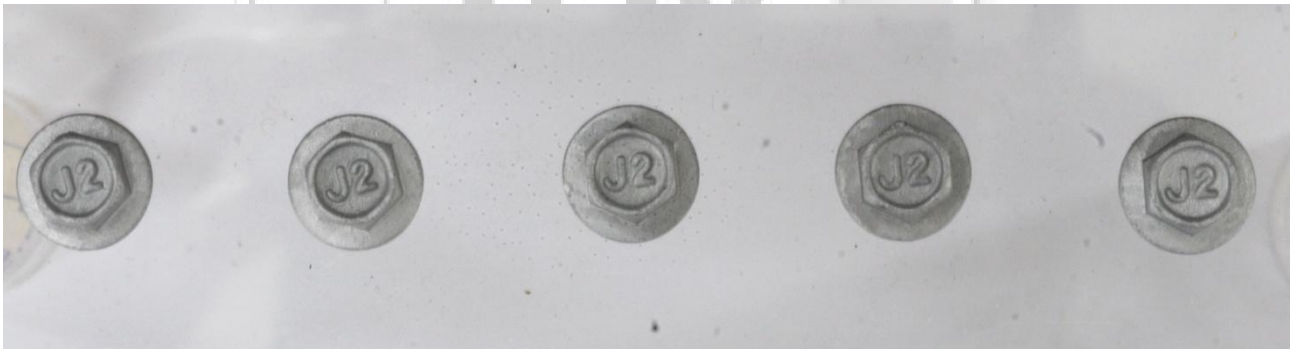
Figure 5. After 2,000 hours of Cyclic Fluorescent UV Lights and Water Condensation Test
