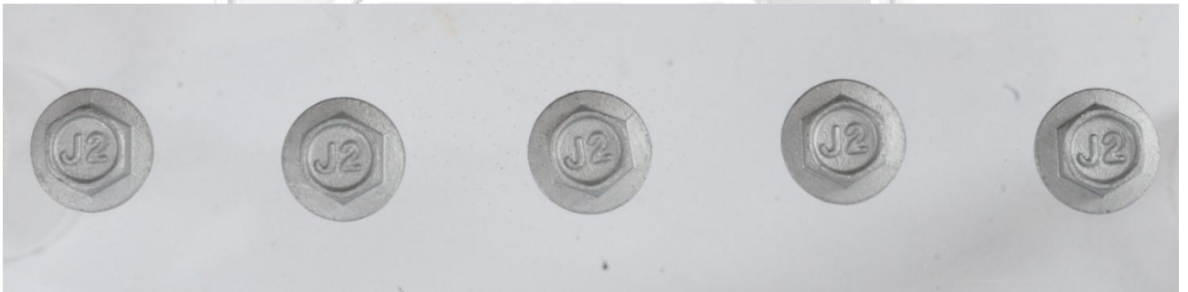
Figure 2. After 500 hours of Cyclic Fluorescent UV Lights and Water Condensation Test
